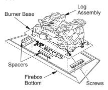
Figure 30 - Removing/Installing Burner Base
